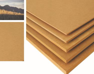
Medium-density fibreboard (MDF) is a wood product valued for its fabricability which allows precision joinery work and finishing. Medium Density Fibreboard is widely used to manufacture furniture. Medium Density Fibreboard can also be used as a building material. Medium Density Fibreboard panels are composed of wood, resin and wax.
